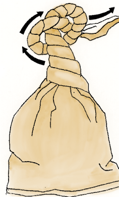
Figure 12D: Tie an overhand knot (pretzel knot) as low as possible on the bag.
