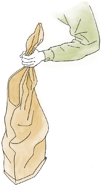
Figure 12A: Sandbag filled 1/4 to 1/3 full
