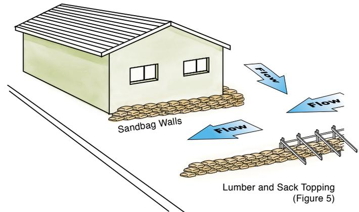
Figure 15: To divert mud, debris, and water, use sandbag walls or lumber and sack topping
