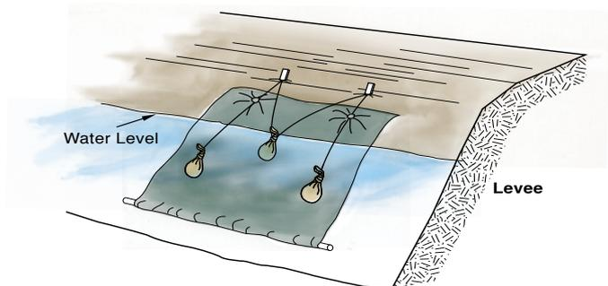
Figure 9: Waterside boil protection
