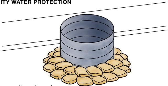
Use sandbags to seal pipe to pavement.
