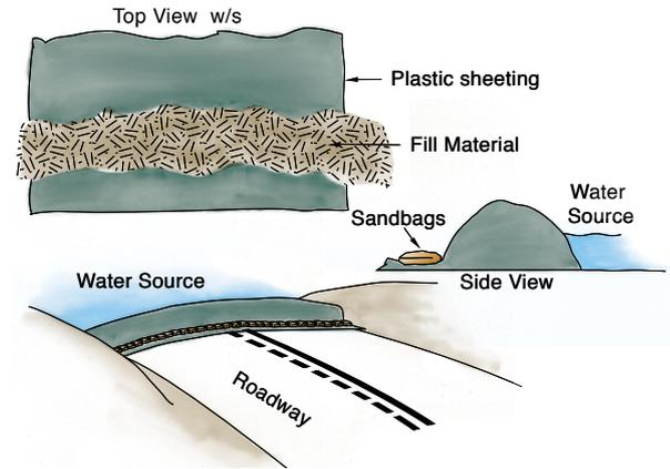
Figure 4: Temporary levee
