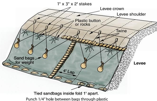
Figure 10: Wavewash Protection
