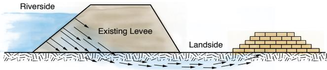
Figure 7: Flow of water through a levee
